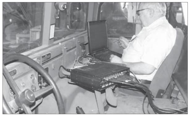
A definite advantage for vehicle test engineers is IOtech WaveBook's ability to operate from the 12-VDC vehicle power supply. The feature lets the equipment run live road tests while operators observe and record data in real time and make necessary vehicle adjustments on the fly.
